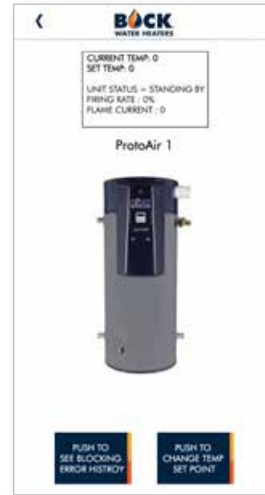
Monitor Current Temp/ Setpoint and Heater Status
